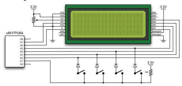
The LCD used in this code example is the NewHaven Display 3.3V 4x20 Display (Digi-Key part #NHD-0420H1Z-FL-GBW-33V3-ND). The code can easily be adapted for other LCD displays.
